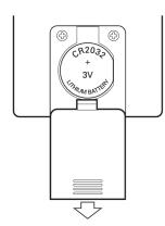
Remove the Battery Compartment Cover.
