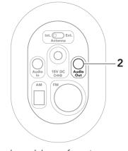
**Note:** Since clearance from the connector to the table surface is minimal, it is suggested that you use a cable with a right angle connector. If you do not have a right angle connector, one may be purchased on **versaudio.com**.
