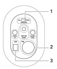
Vers 1.5R is equipped with internal AM & FM antennas for normal use. If improved radio reception is desired, first slide the Antenna switch on the bottom from **Internal** to **External** (1) and attach the appropriate antenna cable to the correct connector; FM (2), AM (3).
